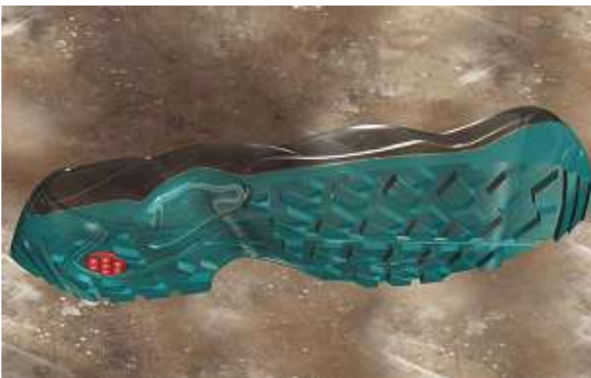
3-D sole model on the CAD
