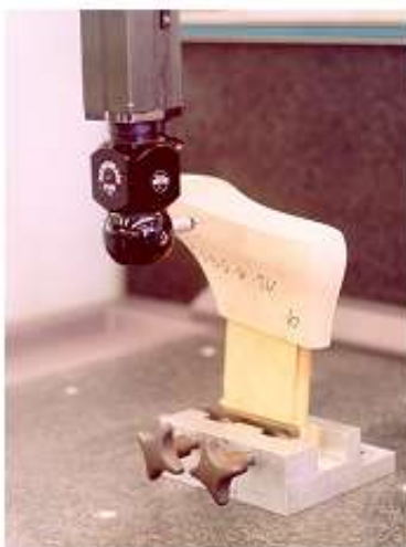
Digital measuring of the last
