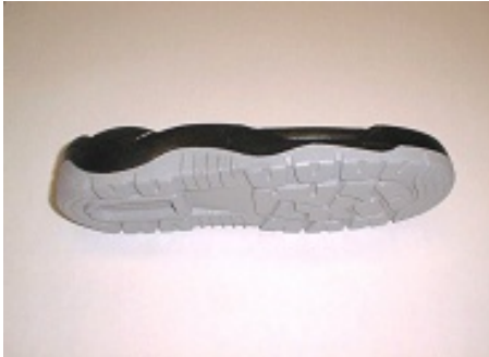
Fig.1: Model sole from the 3D-CAD data
