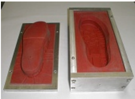
Fig.2: Upper core- and lower cavity plate of Silicone of one-way sample mould
