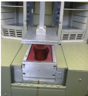
Fig. 3: One-way Silicone sample mould Installed on Lab- or test machine
